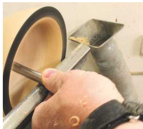
▲ Pic.3 This is my preferred grip when using this tool. My left thumb pushes down on the tool during the cut, which means that the tool can be pivoted easily on the toolrest
